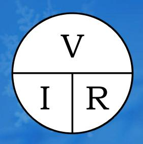
(Voltage = Current \* Resistance) V = 5 Amps \* 0.1 Ohm
